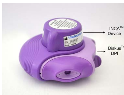
Fig. 1 INCA™ device and functional position on Diskus™ inhaler.
